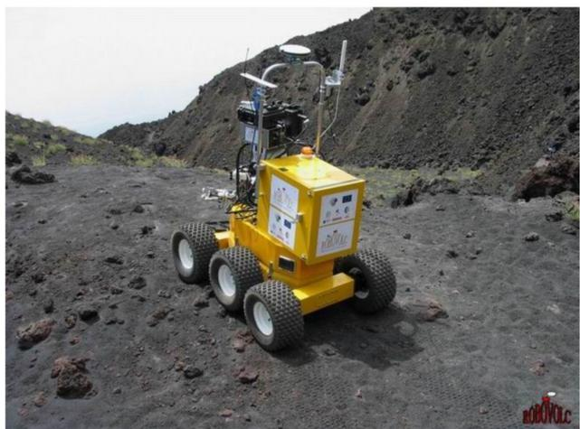
FIGURE 3 – Robot ROBOVOLC
